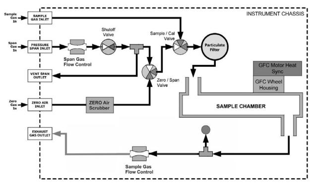
Figure 12-10: Internal Pneumatic Flow OPT 50E – Zero/Span/Shutoff w/ Internal Zero Air Scrubber
